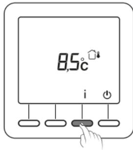
To reset the reading counter, press the C button 3 times.
