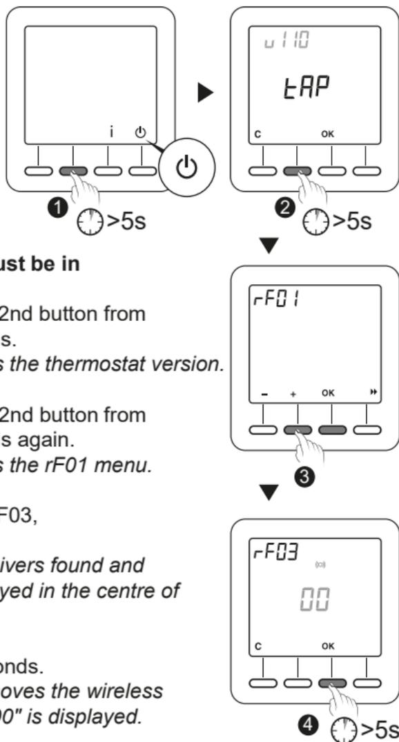
Ê **The thermostat must be in shutdown mode.**
